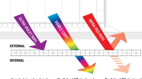
all products in polycarbonate by dott. gallina are UV protected and block out the harmful ultraviolet radiation
